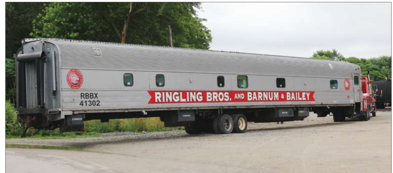
The car is now off the tracks and being pulled by the tow truck. It is being maneuvered in a right angle turn out of the rail yards.
