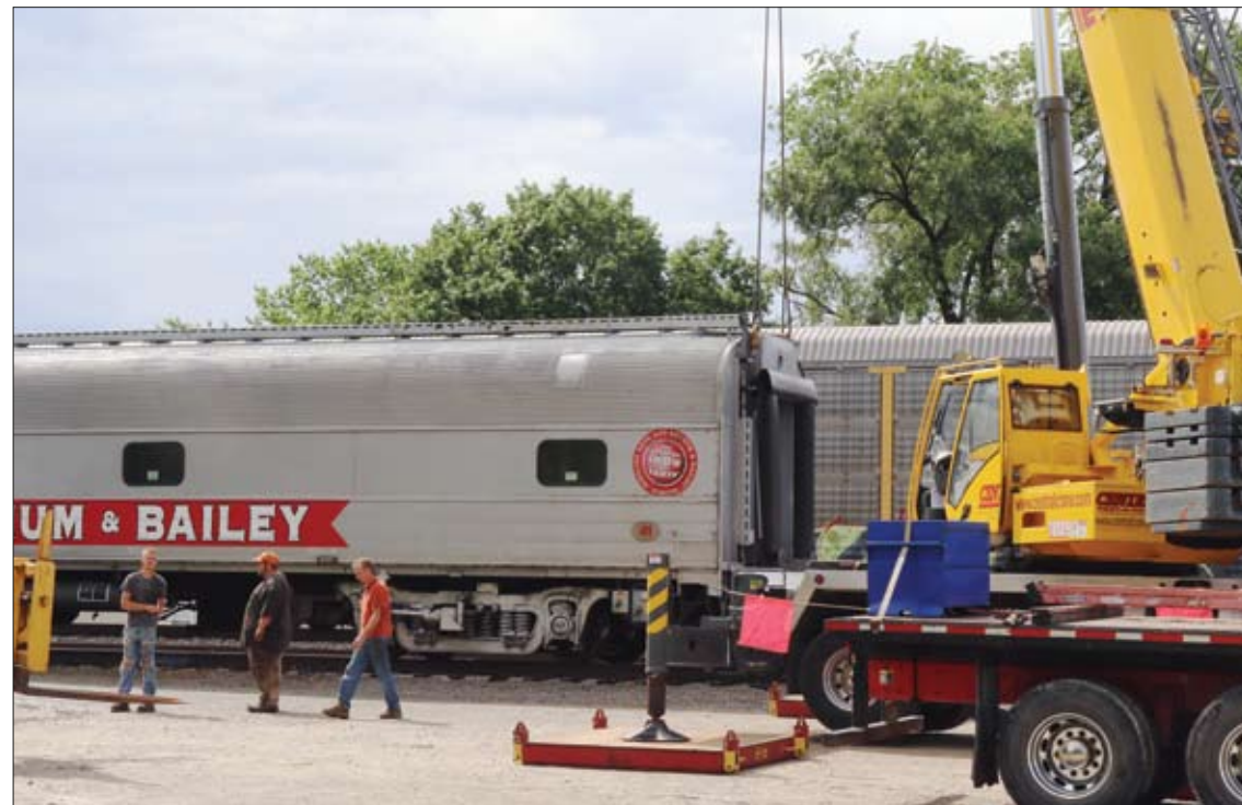
The crane has placed cables onto the train car ready to hoist it up in order to remove the first set of trucks (wheels). Brian Miser is on the right in the red shirt. The flatbed trailer is in the right foreground waiting for the trucks.
